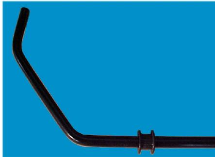
2. Carefully feed the anti-roll bar through the cut out below the upper wishbone front mounting points.
