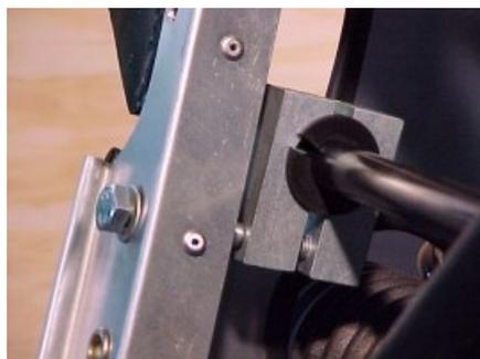
5. Centralise the anti-roll bar to the chassis by ensuring equal distances from the centre point of the bolt heads, securing the rear fixing point of the upper wishbone, to the ends of the anti-roll bar.
