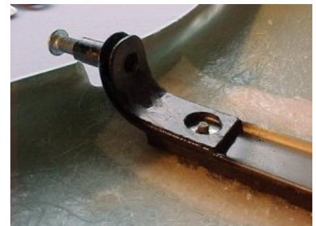
3. After positioning a second M5x20 washer onto the vacant stud, replace a M5 Nyloc nut onto each stud.
