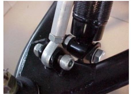
2. Slide the top mounting point of the linkage onto the anti-roll bar until it measures 10mm from the end then tighten the cap screw by hand.
