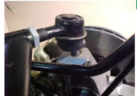
6. Replace the washer followed by the M14 castle nut which must then be tightened until one of its slots aligns with the hole that houses the R-clip. The R-clip must then be inserted.
