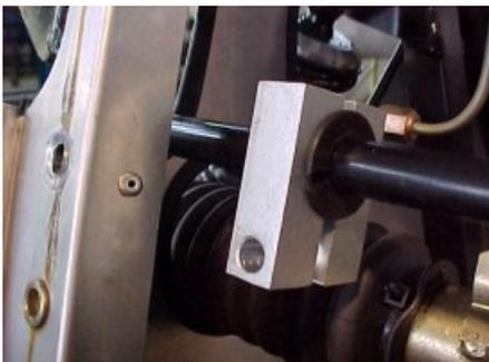
4. Secure both pairs by placing a M8x60 bolt complete with a washer through the chassis and the non-threaded bolt hole of the first block. Rotate the bolt into the threaded bolt hole of the second block but do not fully tighten.
