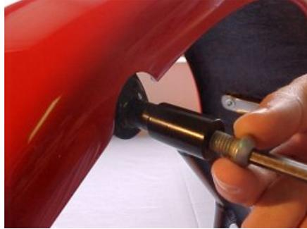
**6.** Tighten all the M5 Nyloc nuts under the cycle fender until the thread protrudes the top of the nut by 1mm.
