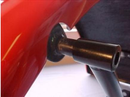
**5.** Using a 5mm allen key, replace and tighten the domehead screws.
