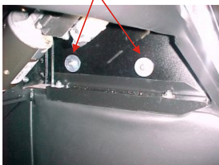
Nuts and washers securing the brackets to the inside of the scuttle
